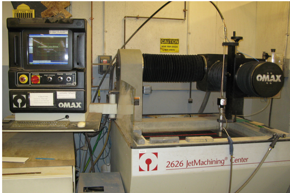
Figure C-1: The Omax 2626 Waterjet cutting machine, maintained by the MIT Hobby Shop, that was used to fabricate the parts for the fluxball machine.
